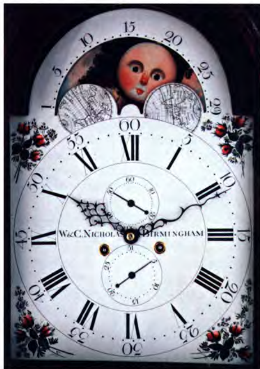
Fig. 24. Moon dial signed for W. & C. Nicholas, Birmingham. The maps, although restored, are basically those used by Ashwin and then Byrne. This dial has a brass falseplate signed 'Ashwin & Co', Allan Smith.
