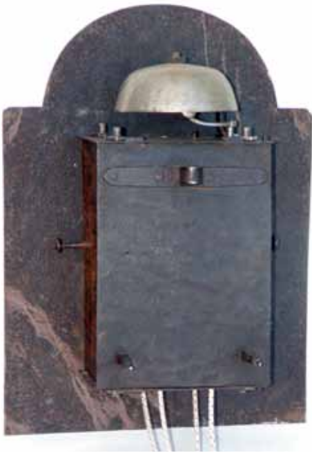
Rear of dial and case showing the hanging hoop, and spikes, with the bell fitted to the top of the case.
