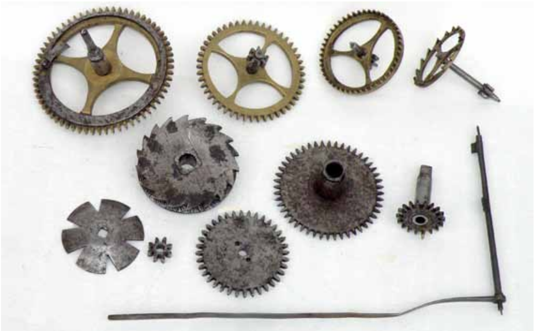
The brass wheels of the going train, the iron motion-work and verge pallets.
