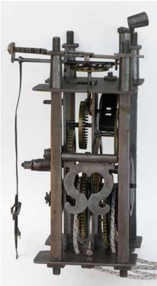
Right-hand side showing the single arbor for the strike-work and the large decorative trip lever.
