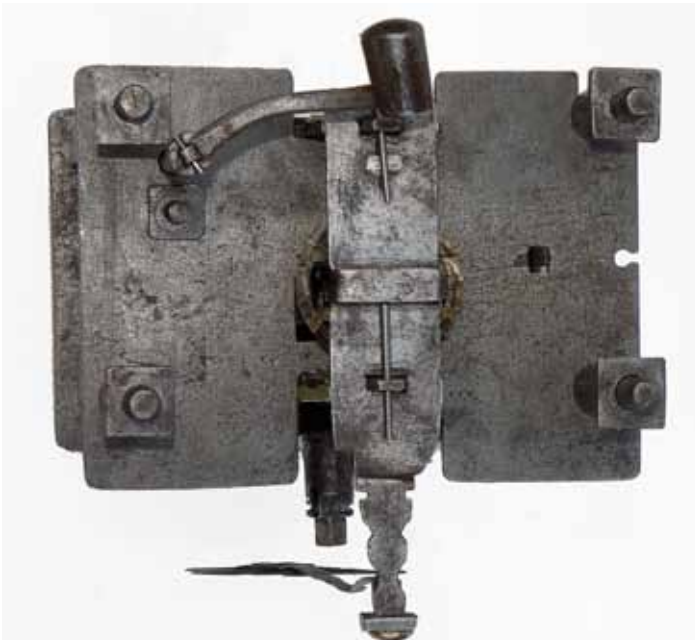
Right-hand side showing the single arbor for the strike-work and the large decorative trip lever.
