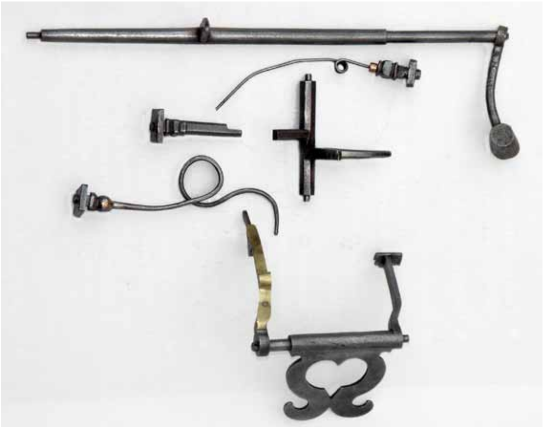
The components of the strike-work, all of iron apart from the brass return spring of the nag's head. The seemingly simple locking detent also acts as an overlift lever and countwheel detent.
