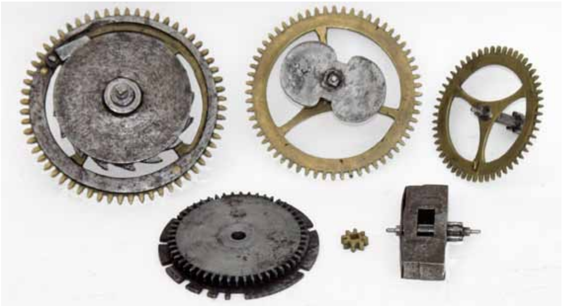
The brass wheels of the striking train, the iron countwheel and its gear wheel, and the very thick iron fly. The 'double heart' on the arbor of the second wheel provides overlift for the nag's head strike.
