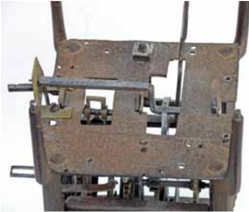
Fig 8 (left) . Top plate showing the later anchor escapement with its cranked pallet arbor.
