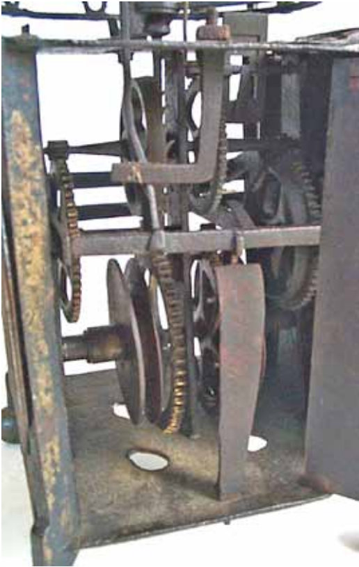
Fig 2. Side view of the movement with brass wheels and iron movement bars. (J. Hooper)
