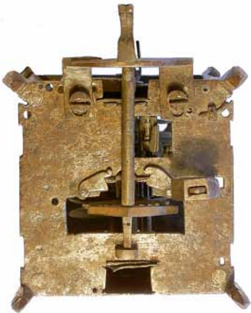
Fig 25. Iron top plate and the later anchor escapement. Note the very unusual use of latches. (M. Hurst)
