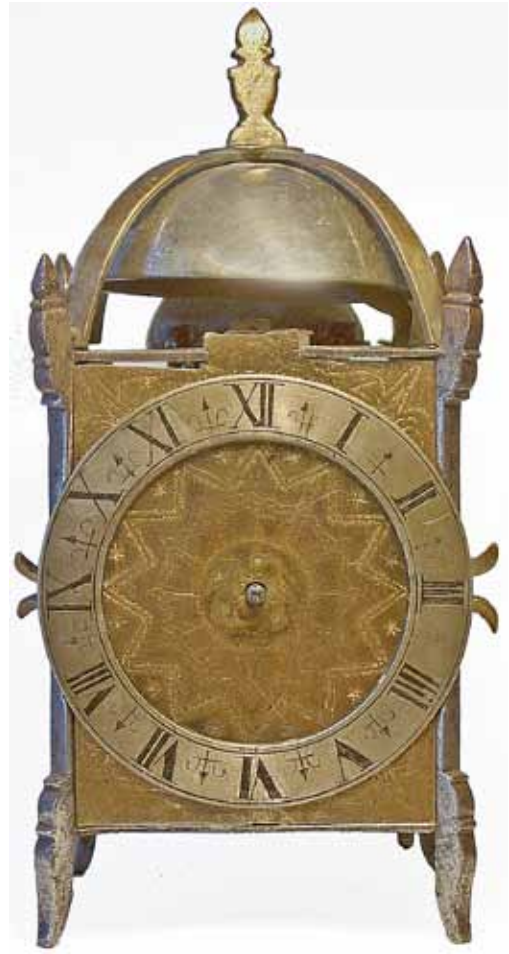
Fig 21. Clock 7. Miniature lantern clock with an iron frame. No frets. (M. Hurst)
