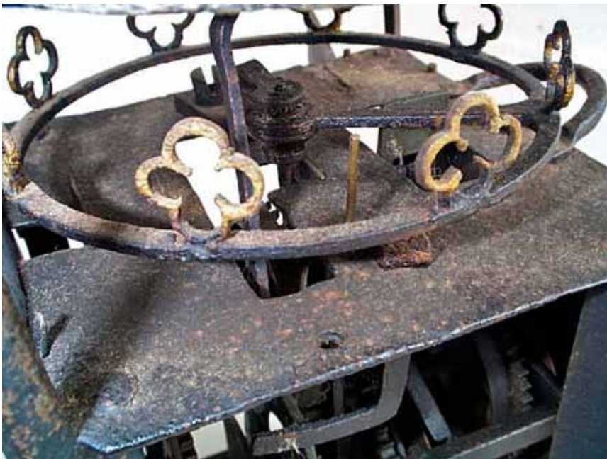
Fig 3. Close-up of the single-spoked iron balance with eight brass quatrefoil attachments. The hoop for hanging the clock on a wall can be seen to the right. (J. Hooper)
