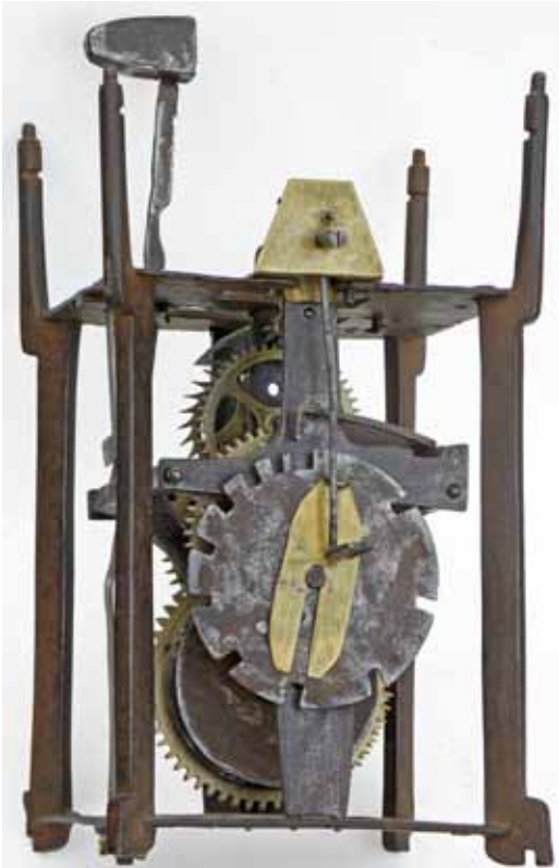
Fig 6. Movement from the rear showing the iron countwheel.
