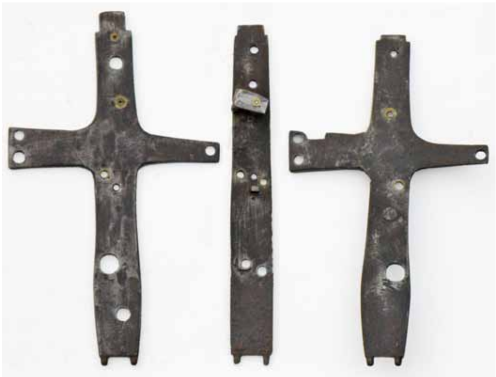
Fig 10 (left). The English-style iron movement bars viewed from the front. Left to right: front, centre, rear. The two large holes near the top and bottom of the front bar are for the later brass dial.
