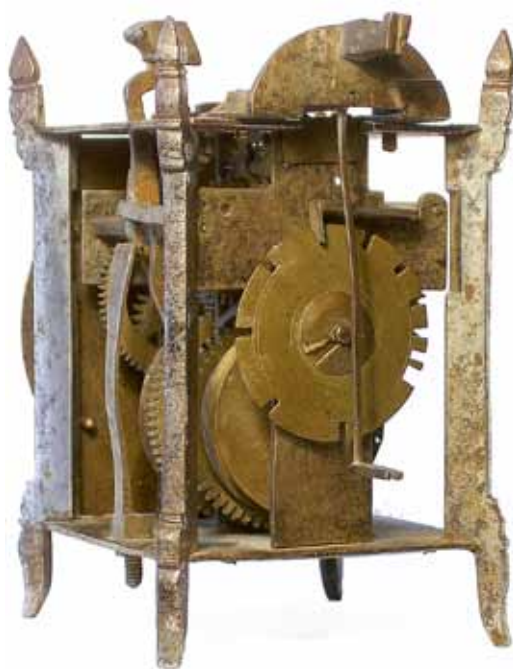
Fig 24. Rear view showing the brass countwheel. (M. Hurst)
