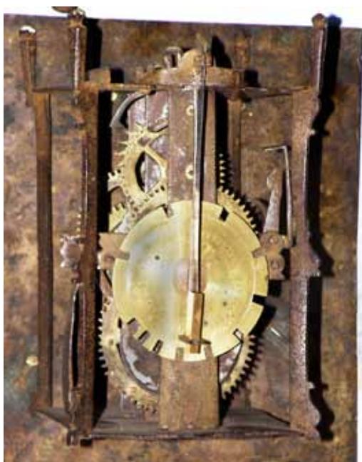
Fig 15. Rear of the movement. Note the 'noses' on the rear corner posts.
