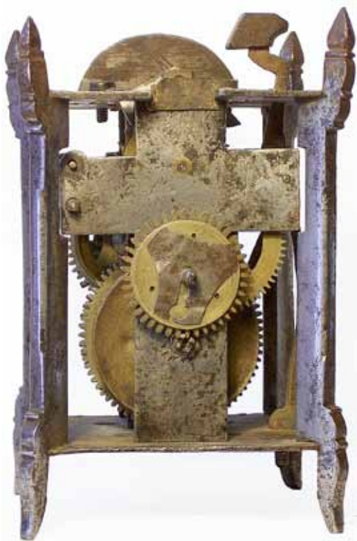
Fig 23. Front view of the movement with iron movement bars. (M. Hurst)
