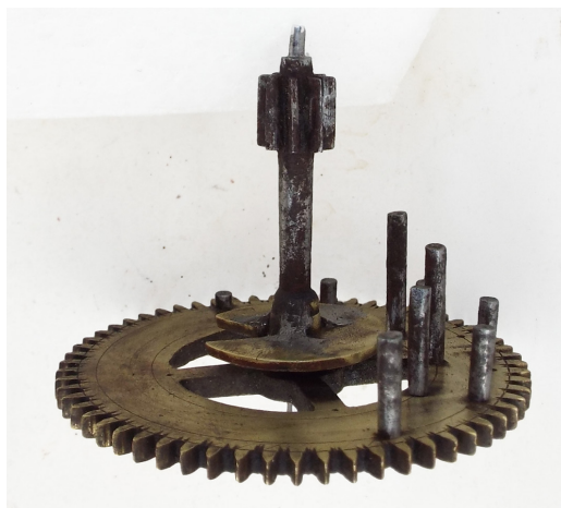
Fig. 24. Clock 4, the pinwheel with hammer pins of graduated lengths: six shorter hour pins and three longer quarter pins.
