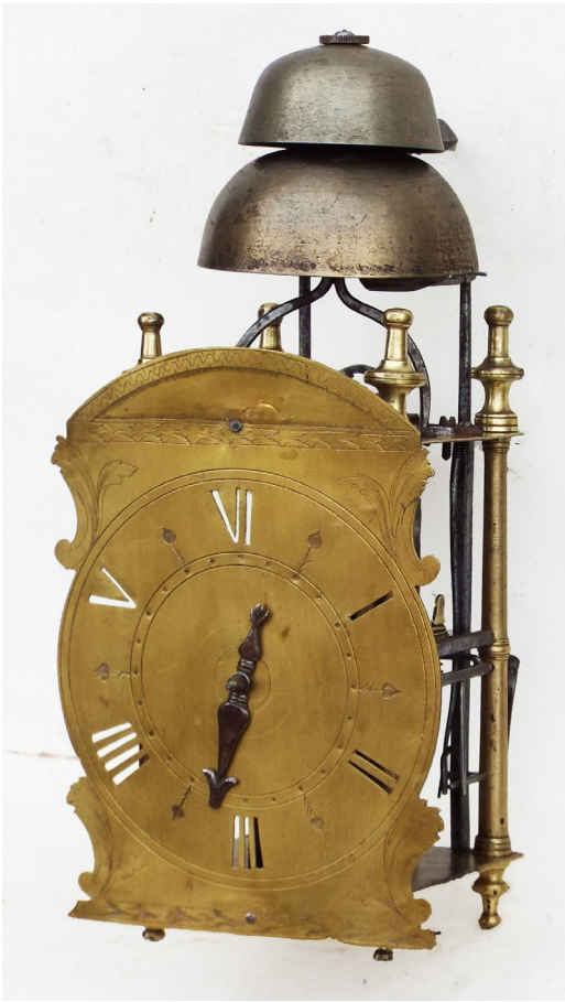
Fig. 19. Clock 4, single-handed clock with whizzing work.
