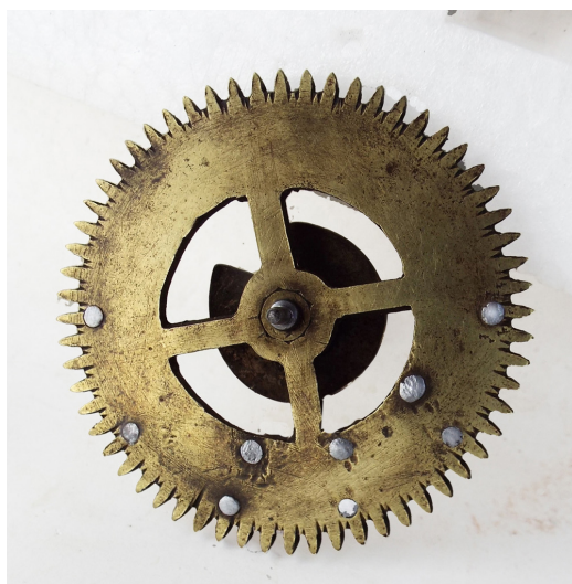
Fig. 23. Clock 4, rear of the pinwheel (striking second wheel) with six outer hammer pins for the hours, and three inner pins for the quarters. The overlift disc has a single notch.
