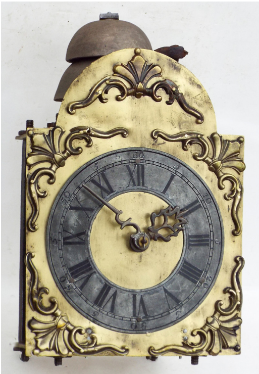
Fig. 13. Clock 3, brass dial with Rococo brass spandrels and an unusual painted pewter chapter ring.
