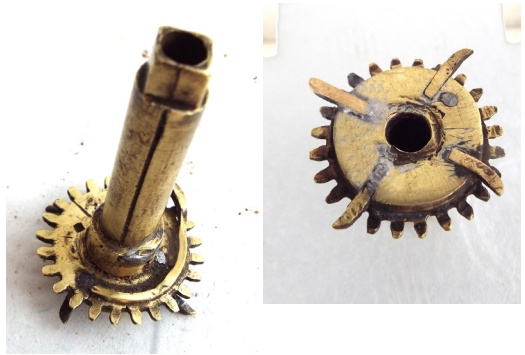
Fig. 15. Clock 3, minute wheel with quarter steps on the front, and four let-off arms at the rear.
