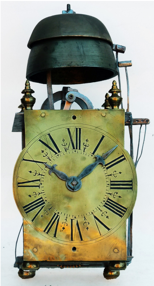
Fig. 8. Clock 2, lantern clock with brass finials and bun feet, with two hands but no minute numbers.
