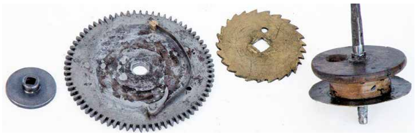
Figure 17. Greatwheel, click wheel, barrel and spacer.
