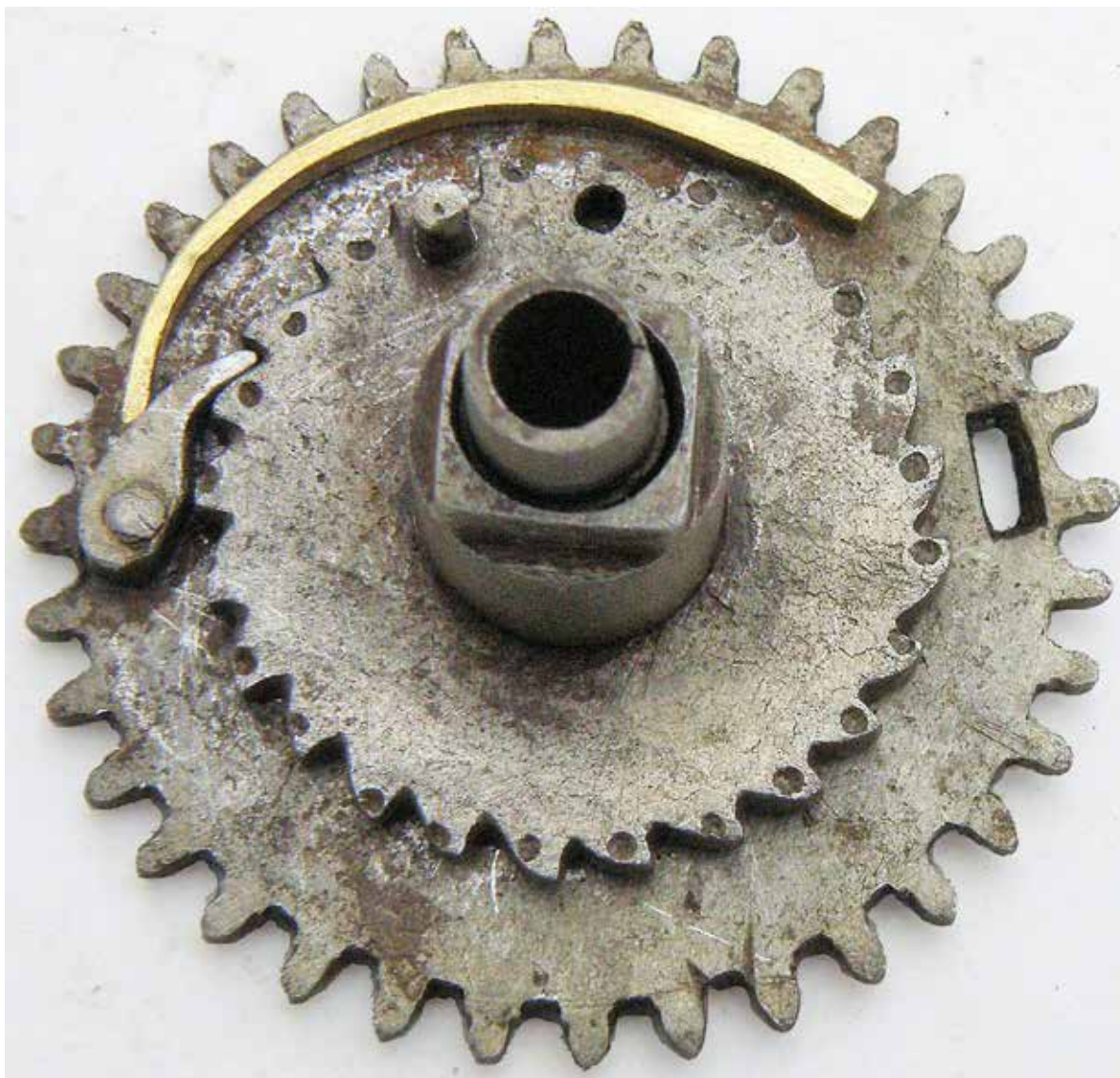
Figure 18. The hour wheel and the ratchet wheel with an alarm let-off pin.
