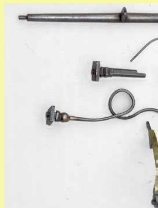
Figure 12. The components of the strikework, all of iron apart from the brass return spring of the nag's head.
