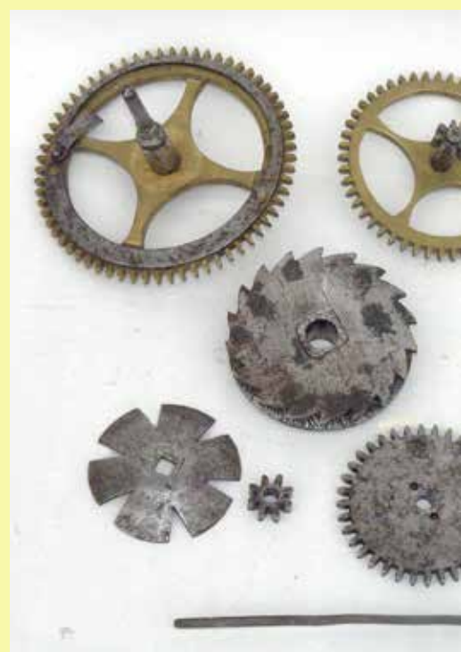
Figure 10. The brass wheels of the going train, the iron
