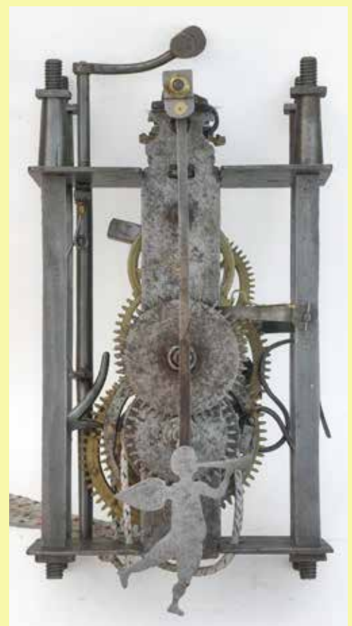
Figure 5. Movement from the front showing the vertical hammer shaft.
