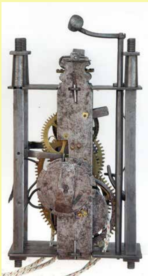
Figure 6. Rear of the movement showing the method of securing the movement bars.
