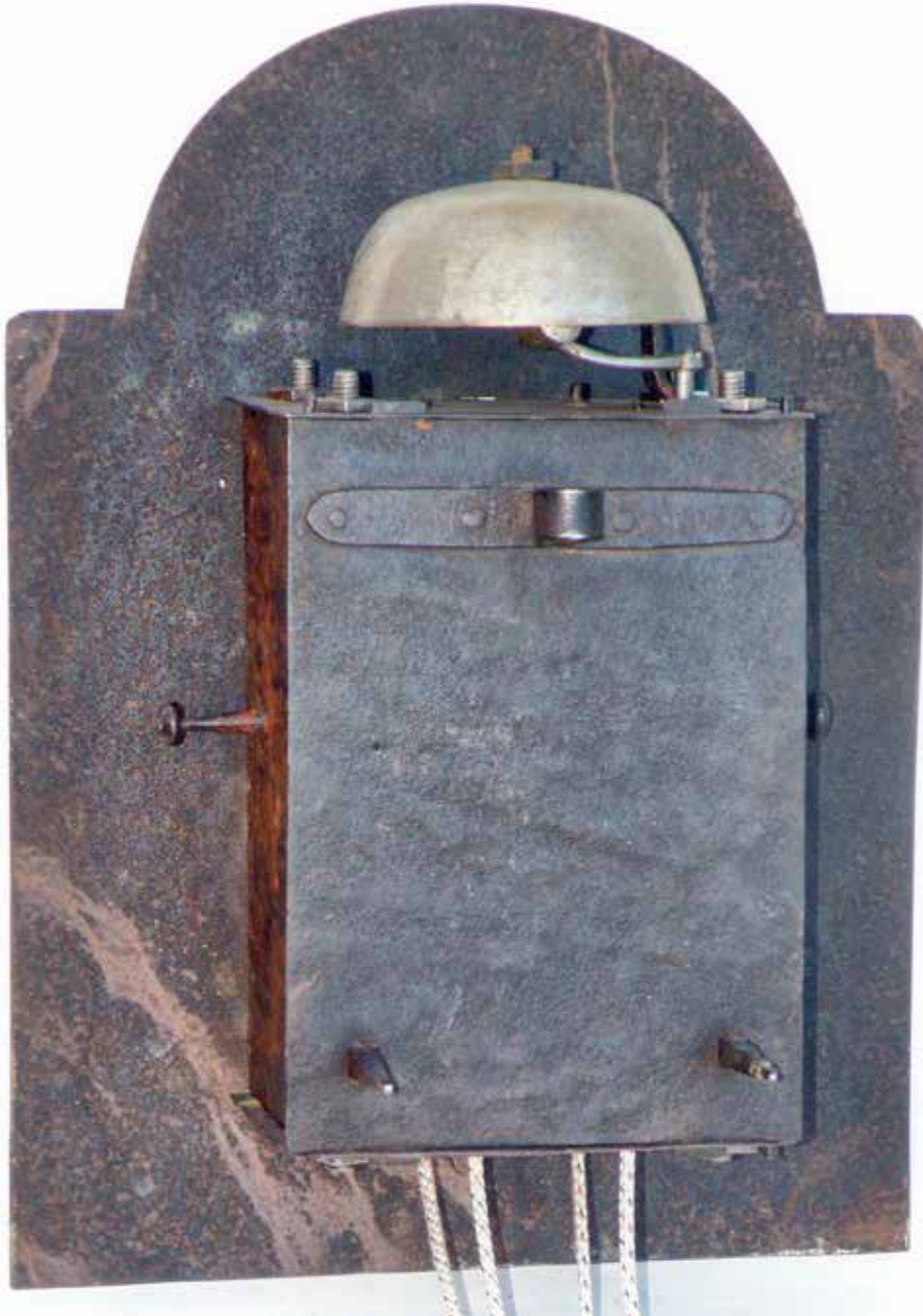
Figure 2. Rear of dial and case showing the hanging hoop and spikes, with the bell fitted to the top of the case.
