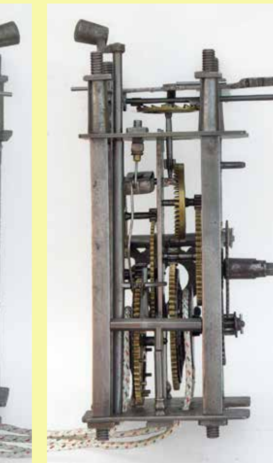
Figure 8. Movement from the left showing the verge escapement.
