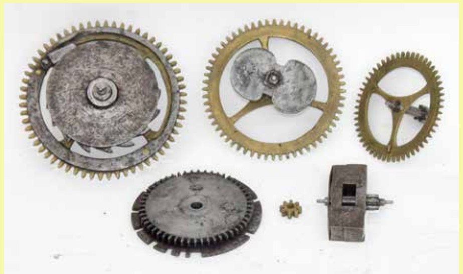
Figure 11. The brass wheels of the striking train, the iron countwheel and its gear wheel, and the very thick iron fly.
