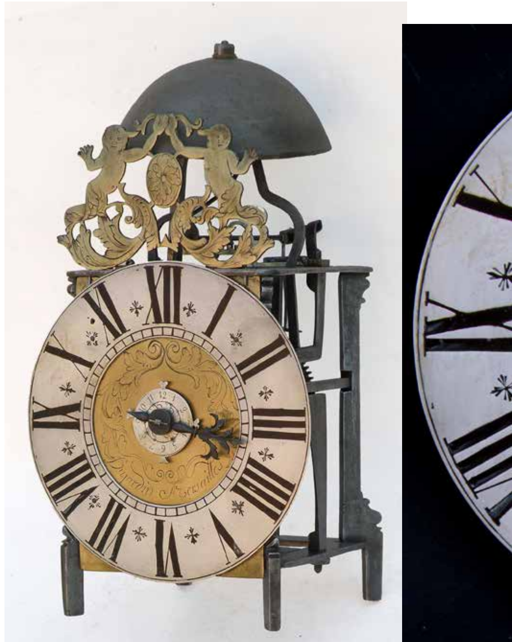
Figure 1. Dujardin clock with a Gothic iron frame.
