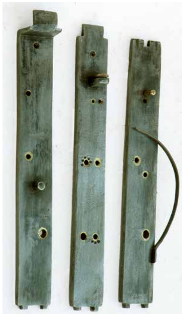
Figure 6. The iron movement bars. The spring for the passing half hours is on the front bar (right).
