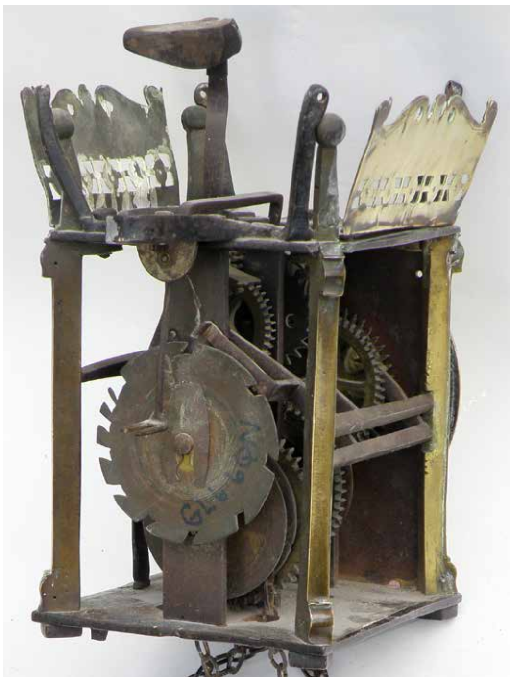
Figure 6. The movement with the strikework and hammer arbors pivoted between typical mid seventeenth-century French Gothic pillars.
