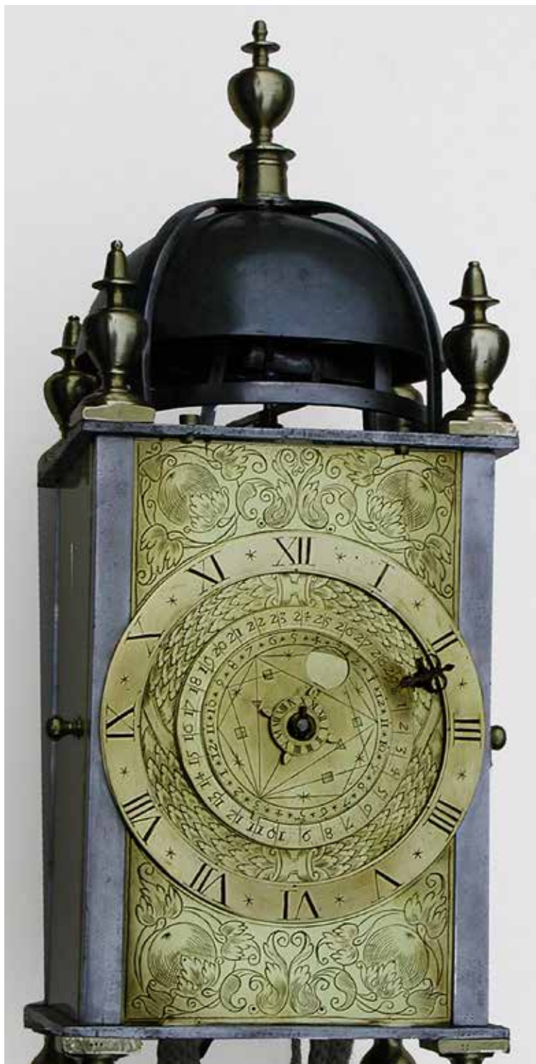
Figure 7. Weight-driven clock with a lunar and astrological dial, iron pillars, plates and movement bars and brass feet and finials (Brian Loomes).
