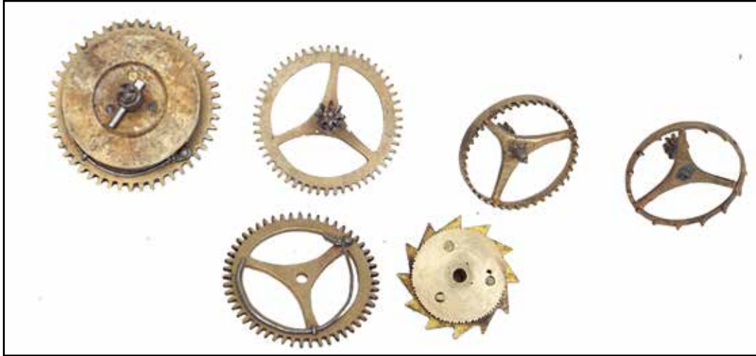
Figure 17. The four wheels of the going train (top) and the special motionwork (below).
