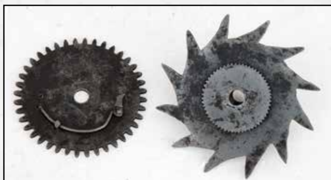
Figure 12 (inset). Hand setting is by a fine-toothed wheel riveted behind the ratch and a click on the hour wheel.
