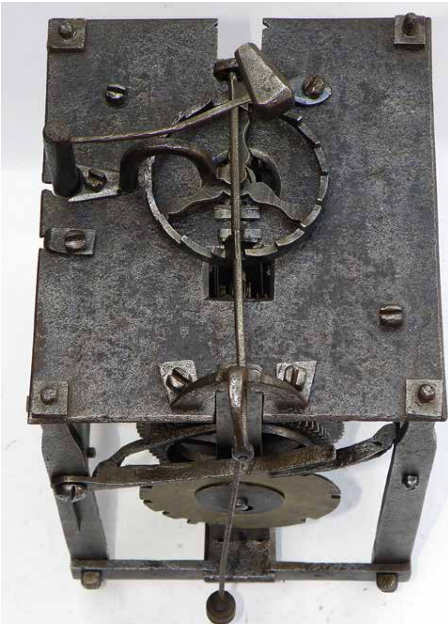
Figure 10. Top of the movement showing the escapement with a large crownwheel and the verge pivoted in a cock and a bridge.
