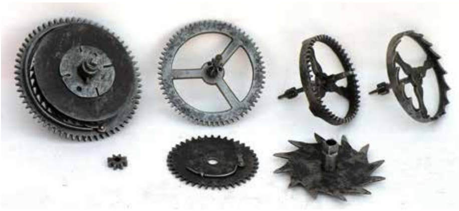
Figure 8. The going train with a separate pinion of report.
