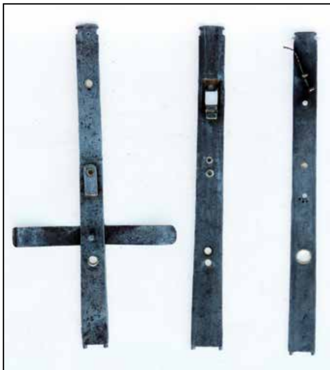
Figure 5. The iron movement bars. Note the clearance aperture in the central bar for the crownwheel pinion. The rear bar has spring cross arms to hold the countwheel in place and a cock for the rear pivot of the locking arbor.
