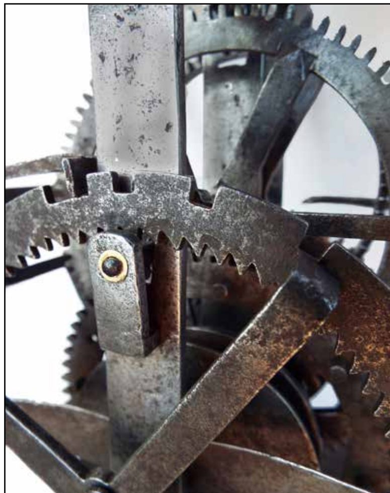
Figure 13. Internal saw-shaped teeth on the countwheel, gathered by a pallet on the rear end of the locking arbor.
