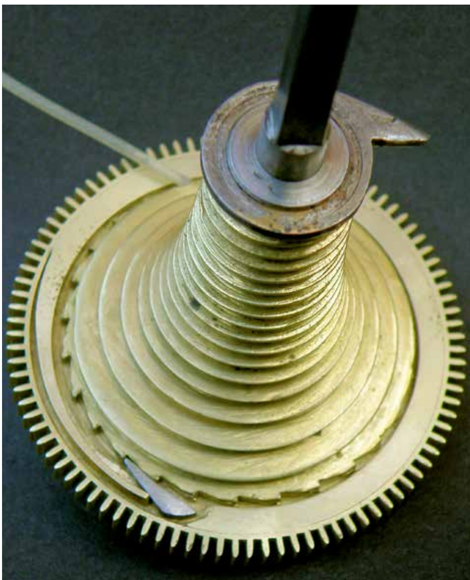
Figure 7. Early type of open fusee with the ratchet teeth cut into the edge of the fusee and the click spring part of the wheel (shown after repair).
