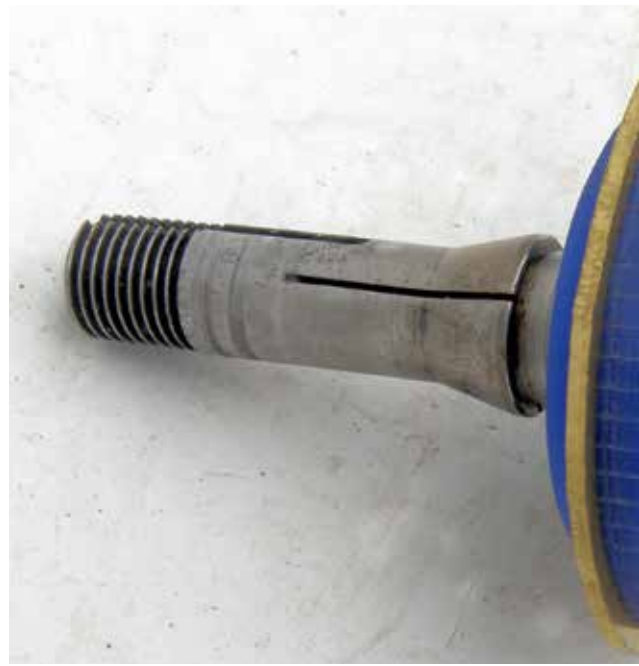
Figure 12. Brass disc held between Perspex backing discs in a mandrel made from an old collet.
