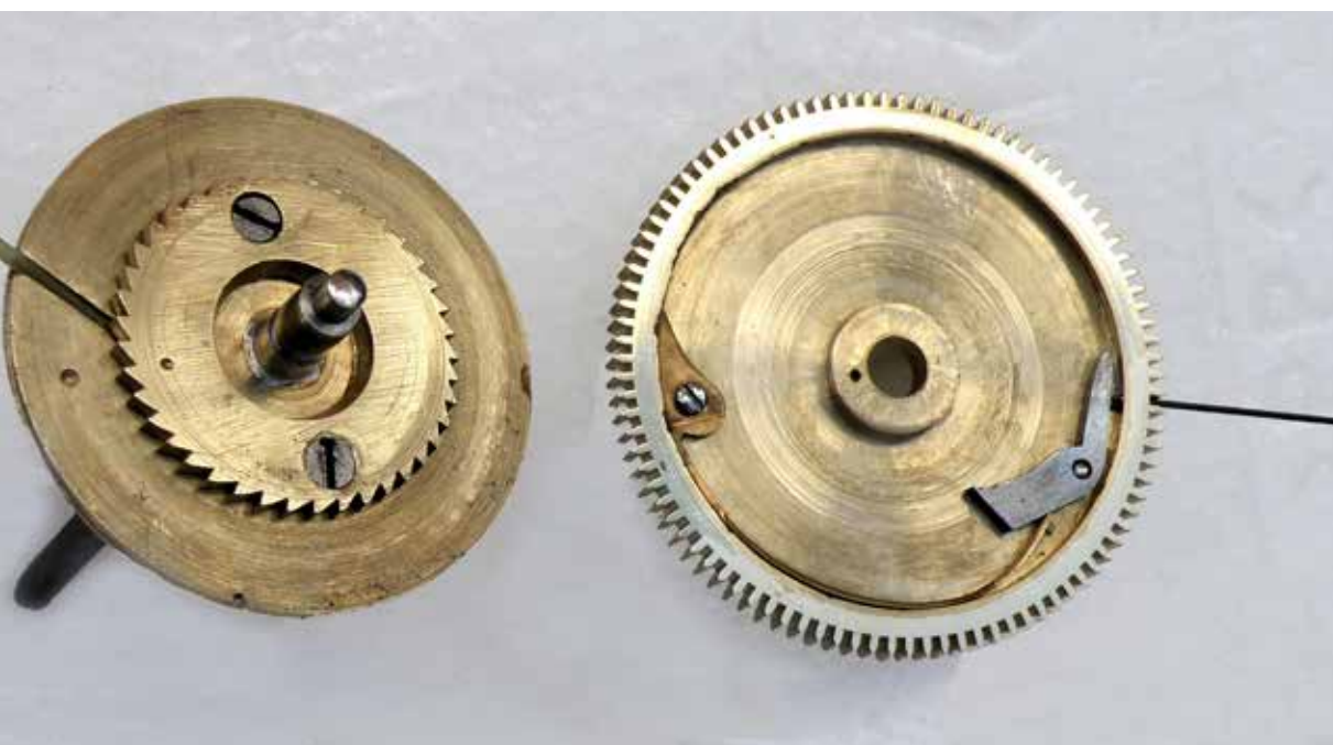
Figure 4 (far left). The enclosed type of fusee used in the nineteenth century.
