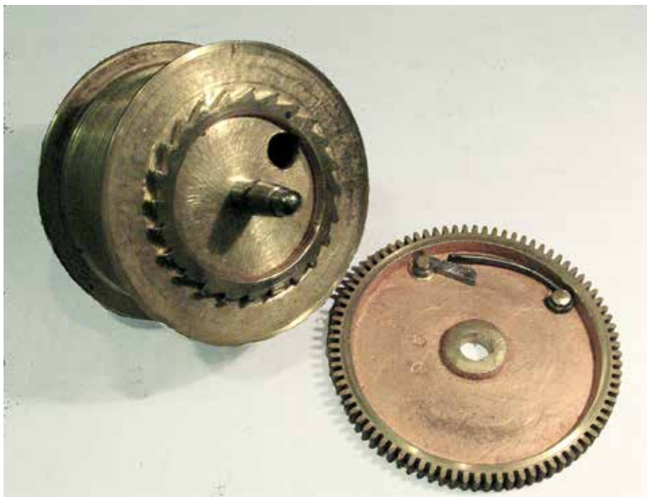
Figure 6. Internal click on the barrel of an eight-day Deacon longcase clock.
