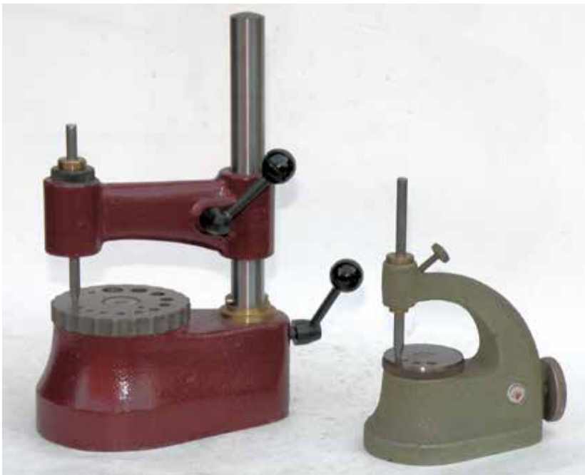
Figure 11. A watchmaker's staking tool (right) and the larger versatile JMW staking tool (left).
