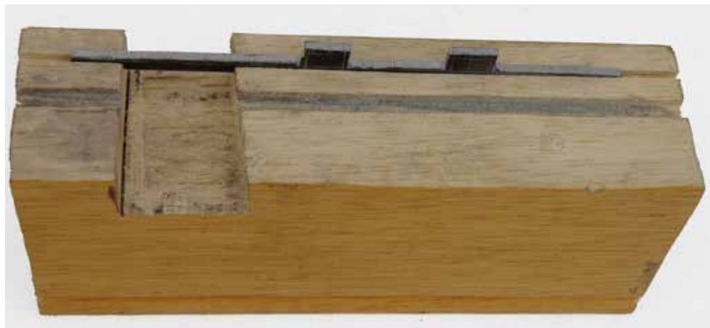
Figure 24. The verge held in a wooden block for filing.
