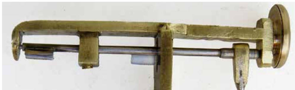
Figure 28. The pivots turned, the pallets shortened and the pendulum fitted.
