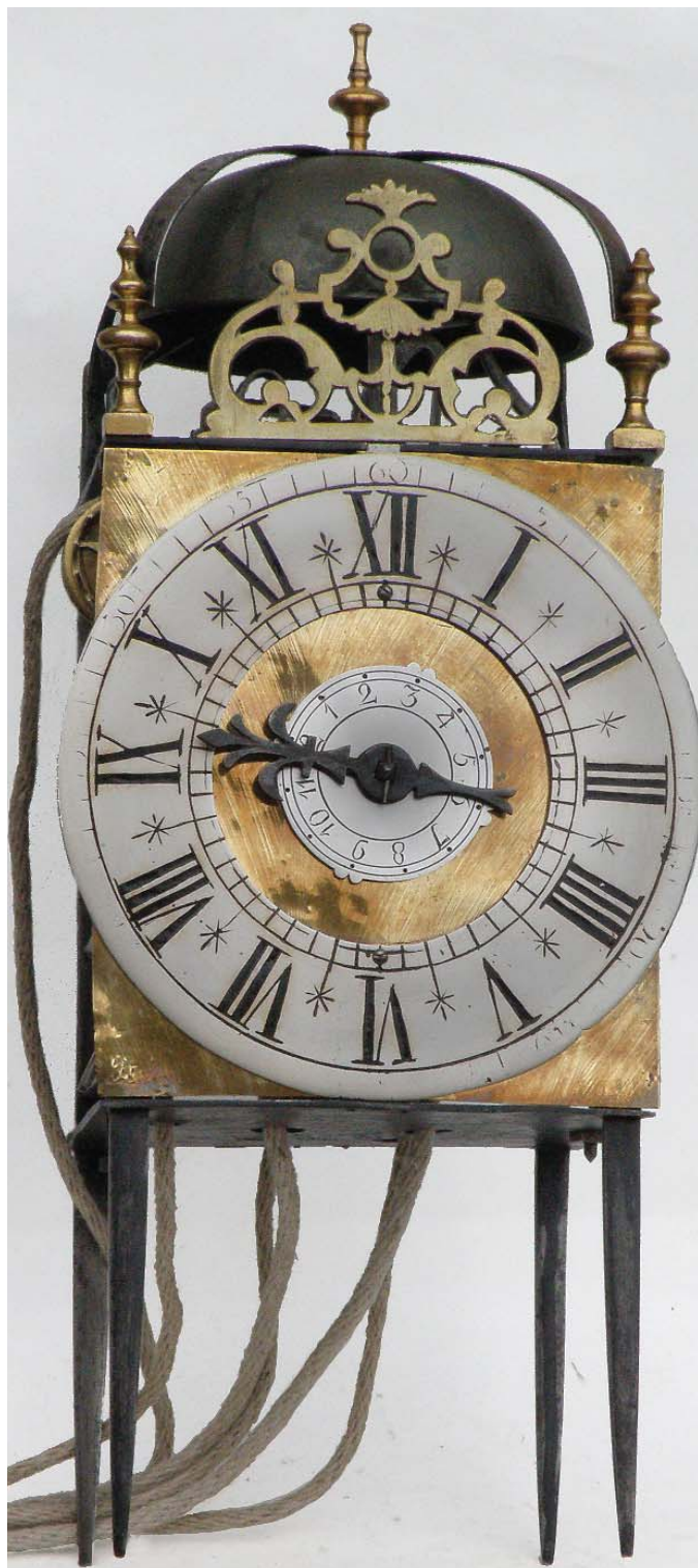
1. Single-handed 8-day French posted-frame clock with restored alarm-setting disc.
