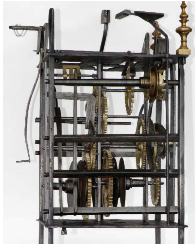
16. The left-hand side showing the crownwheel, lever arbor (second from bottom) and vertical verge of the restored alarm.
