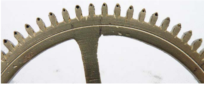
7. Punch marks on the teeth of the going second wheel.
