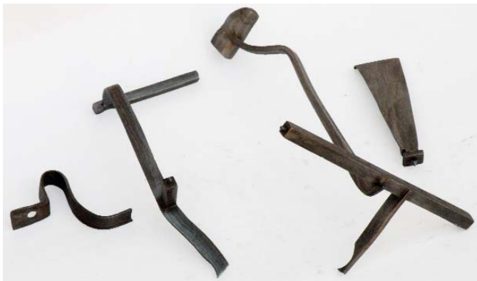
14 The hour hammer and spring (right) and passing half-hour hammer and spring (left).
