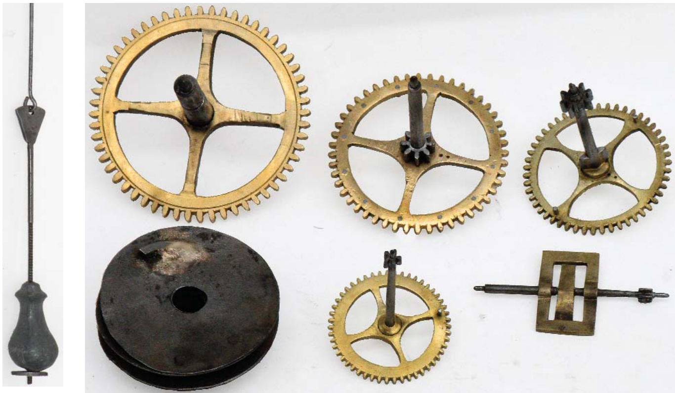
11 The lead pendulum bob. 12. The striking train. Note the two locking pins on the third wheel and the twin gathering pallets filed from the arbor.
