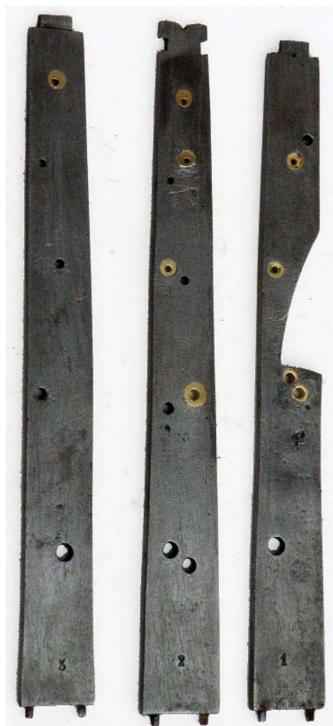
5. Iron movement bars with no side arms and original brass plugs for some of the pivot holes.
