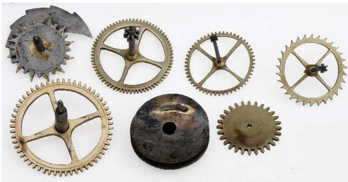
6 The brass wheels of the going train together with the iron hour wheel and iron snail (top left), the iron rope pulley and the large brass pinion-of-report (lower right).
