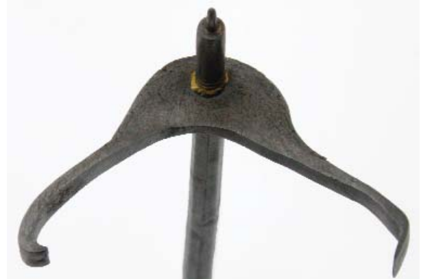
10. The forged-iron anchor pallets.
