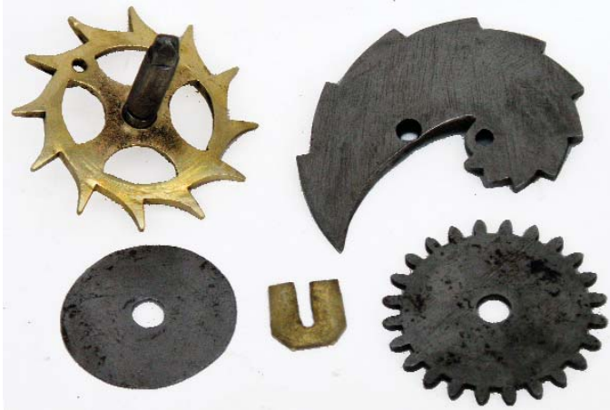
8. Components of the hour wheel, starwheel and snail assembly.
