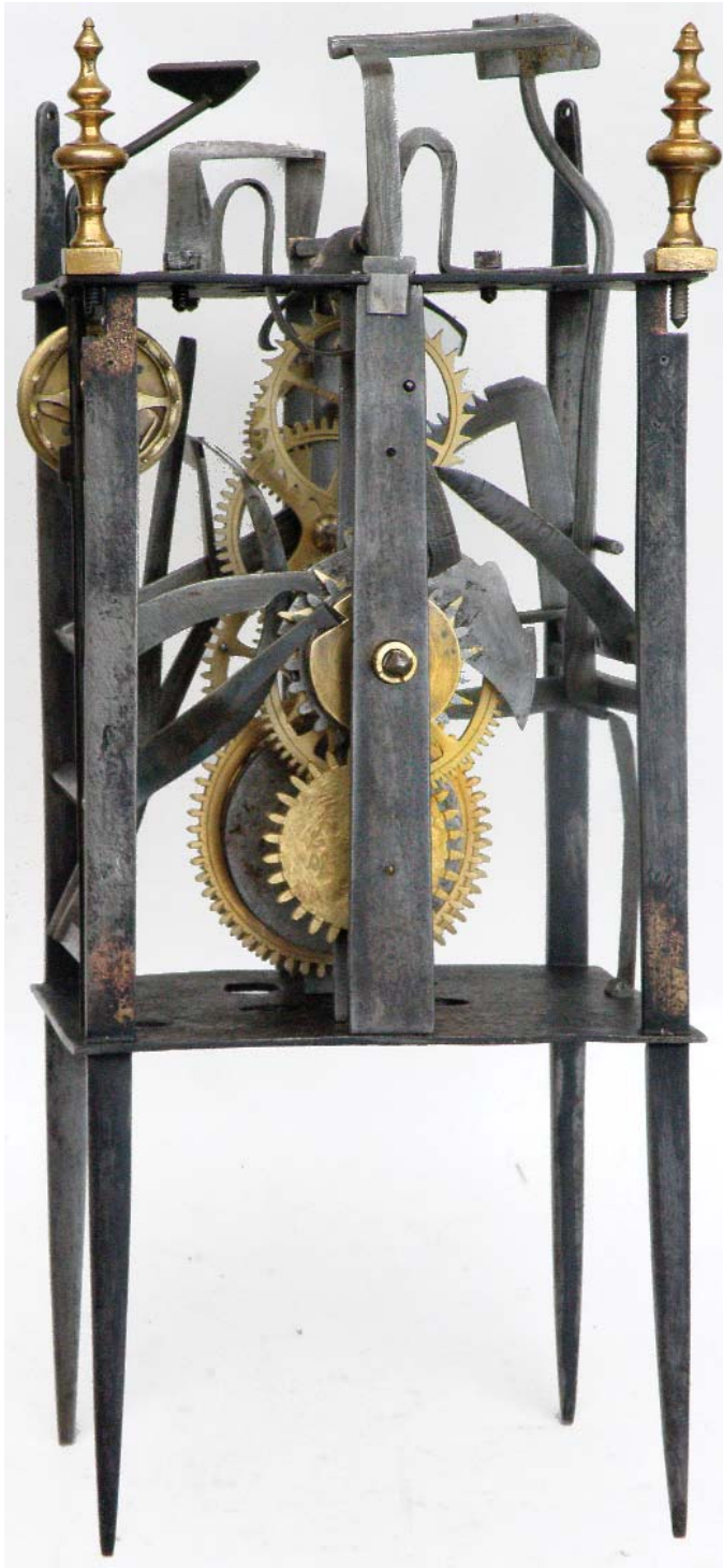
2. The movement from the front with the restored alarm and passing half-hour hammer.
