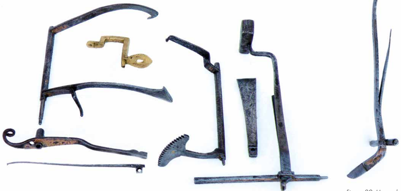
Figure 19. Components of the strike work, including the hammer and hammer spring. Also shown is the crown wheel top cock.
