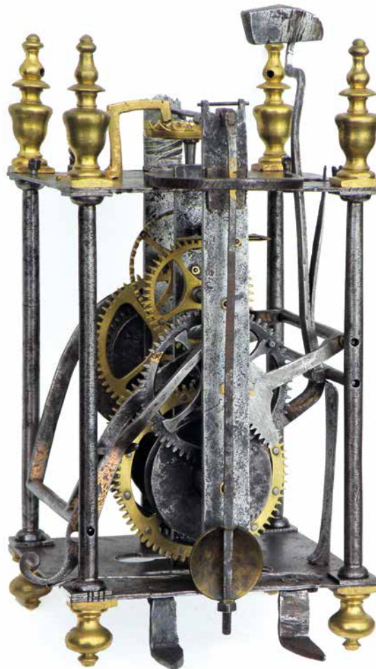
Figure 6. The rear of the movement. Note the knife edge suspension, the rack and the downward cranked spikes.
