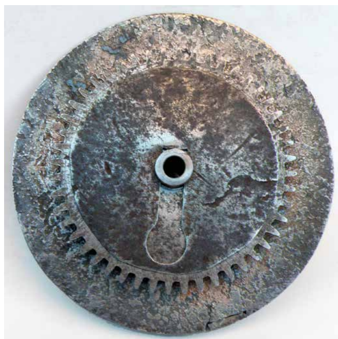
Figure 23. Rear of the motion work with the hour wheel held by the friction spring.
