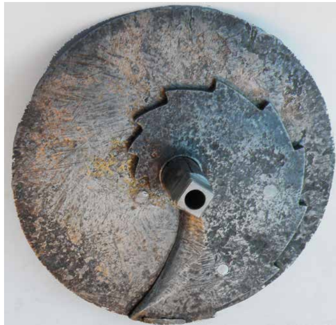
Figure 22. Front of the motion work with the iron snail riveted to the disc.
