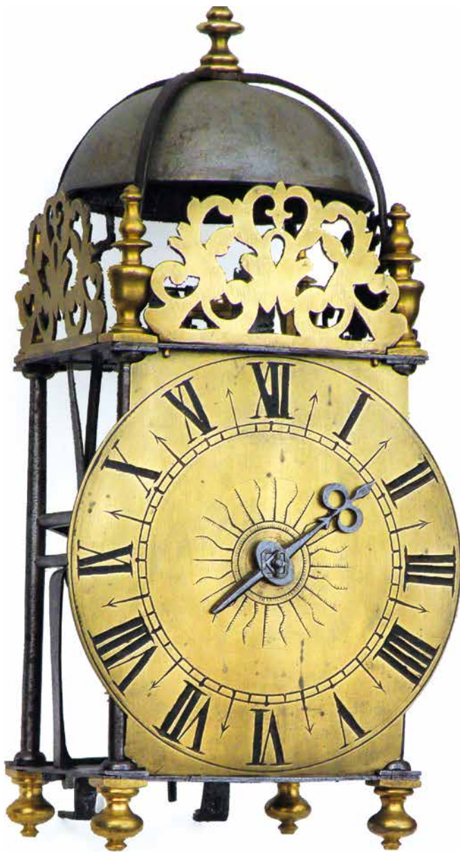
Figure 1. Unsigned French lantern clock with an iron frame and rack striking.
