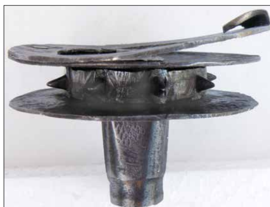
Figures 11 and 12. The rope pulley from the going great wheel with an unusual construction of the click.
