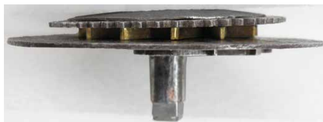
Figure 24. The brass star wheel is hidden between the disc and the hour wheel.
