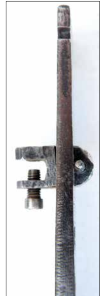
Figure 15. Potence with screw adjustment, fixed to the central movement bar with a taper pin.
