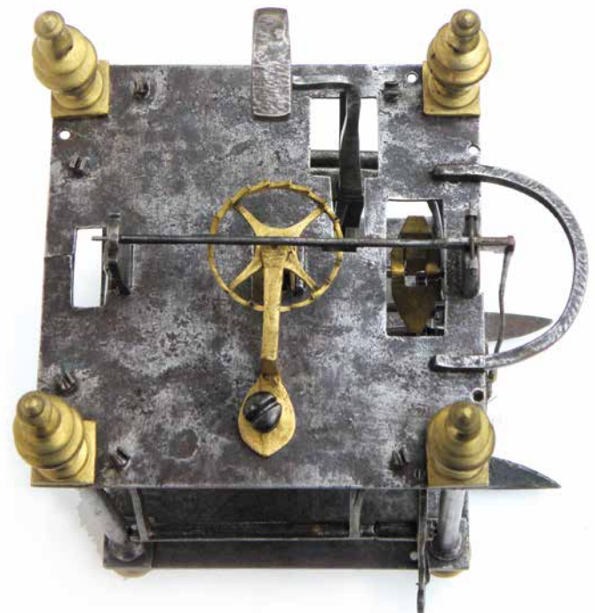
Figure 9. Top view showing the verge escapement.
