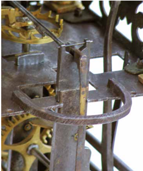
Figure 13. The vee-bed filed in the top of the rear movement bar.
