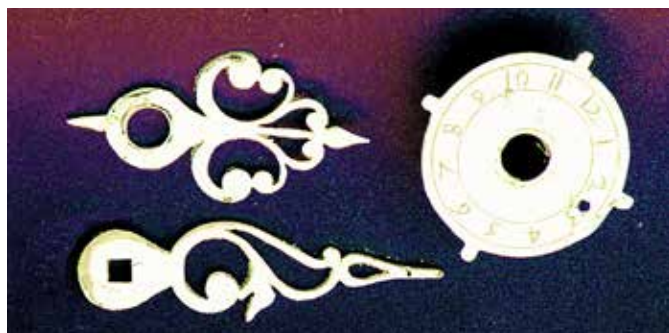
Figure 2. The brass hands and alarm disc.
