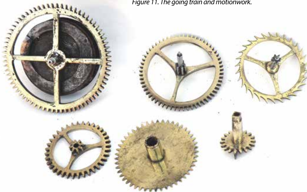
Figure 11. The going train and motionwork.
