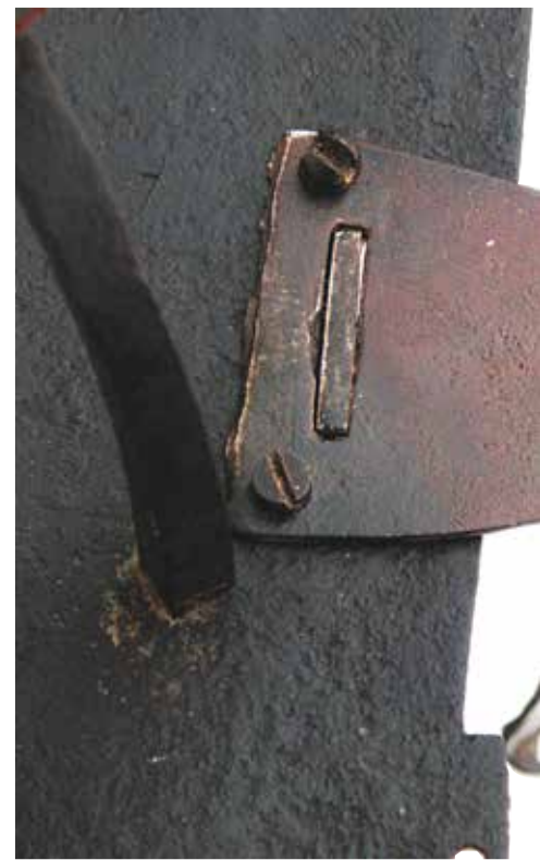
Figure 8. Rear movement bar held by the back cock.
