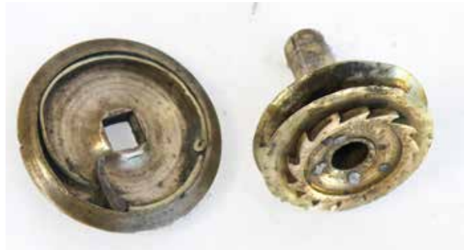
Figure 14. Alternative views of the click and ratchet.
