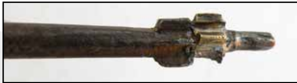
Figure 11. Worn and damaged second pinion.
