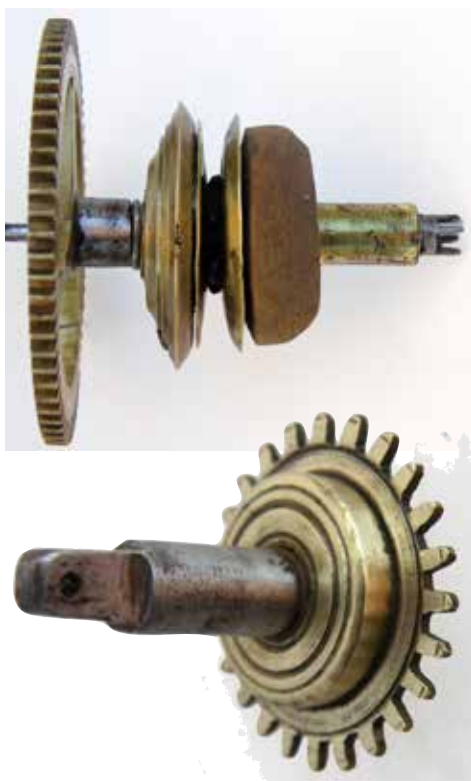
Figure 15 (top left). The pulley and click assembled on the greatwheel arbor. Figure 16 (above left). Hour wheel with brass friction disc. Figure 17 (top right). Brass bush holding the hour wheel against the friction disc. Figure 18 (above right). The alarm pipe, let-off flag and friction disc.
