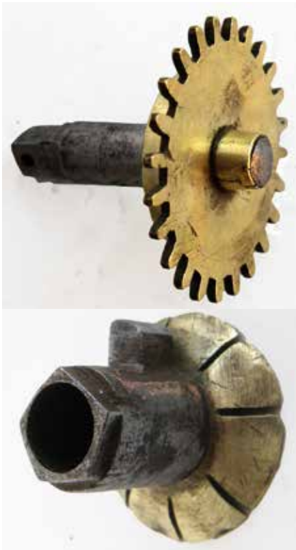
Figure 15 (top left). The pulley and click assembled on the greatwheel arbor. Figure 16 (above left). Hour wheel with brass friction disc. Figure 17 (top right). Brass bush holding the hour wheel against the friction disc. Figure 18 (above right). The alarm pipe, let-off flag and friction disc.
