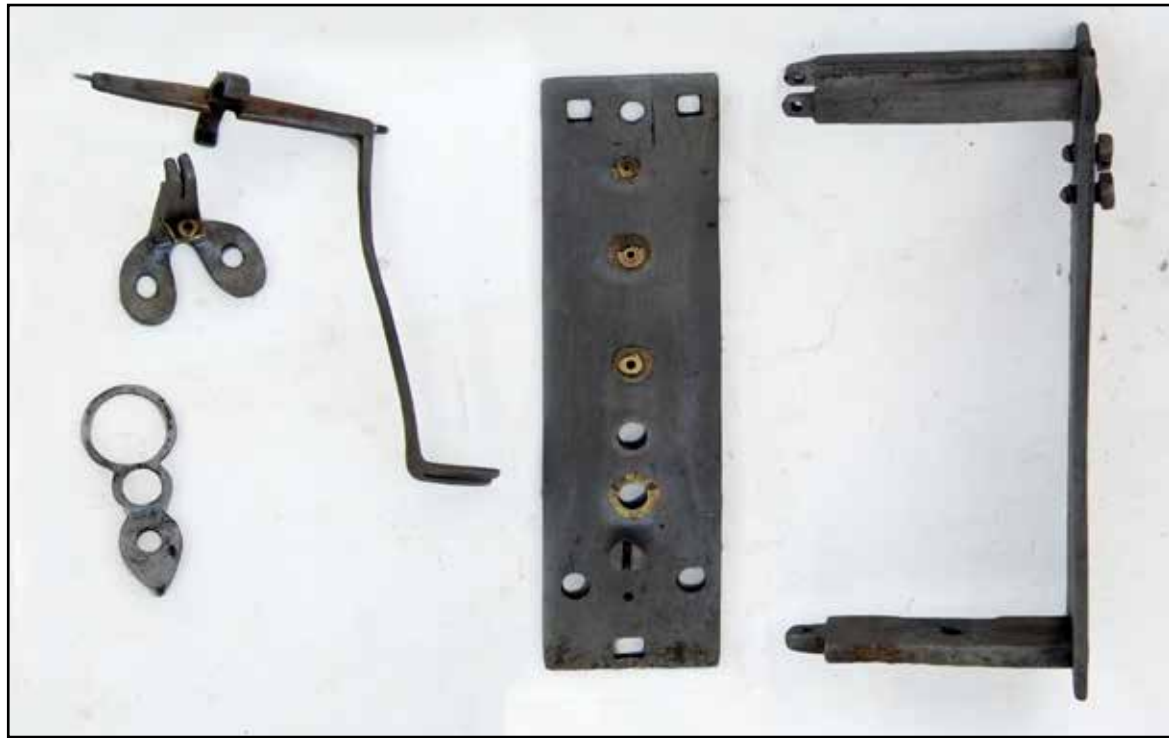
Figure 9. The movement 'plates', anchor, backcock and support for the hour wheel.
