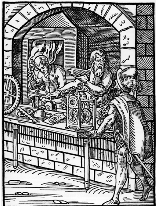
Fig. 30. 'The Clockmaker' by Jost Amman (1568) showing a Gothic clock and another in the course of construction. An assistant hammers an iron plate on an anvil with a forge at the rear.
