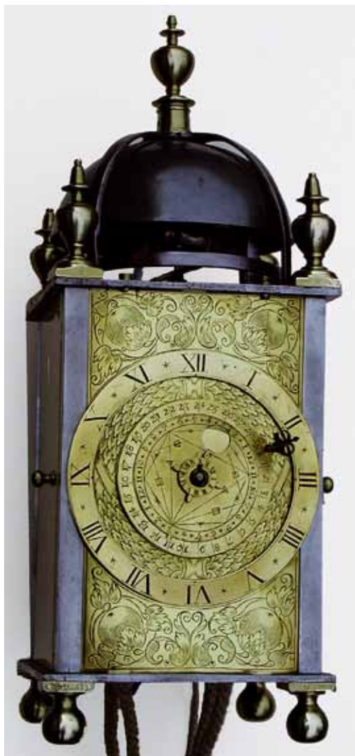
Fig. 13. The so-called 'Precursor clock' with square-section iron pillars, iron plates, lunar and astrological displays. (Brian Loomes)
