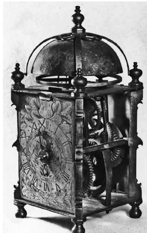
Fig. 23. Movement of the Vallin clock showing the transverse trains with the frame, movement bars and wheels made of iron. (© Trustees of the British Museum)
