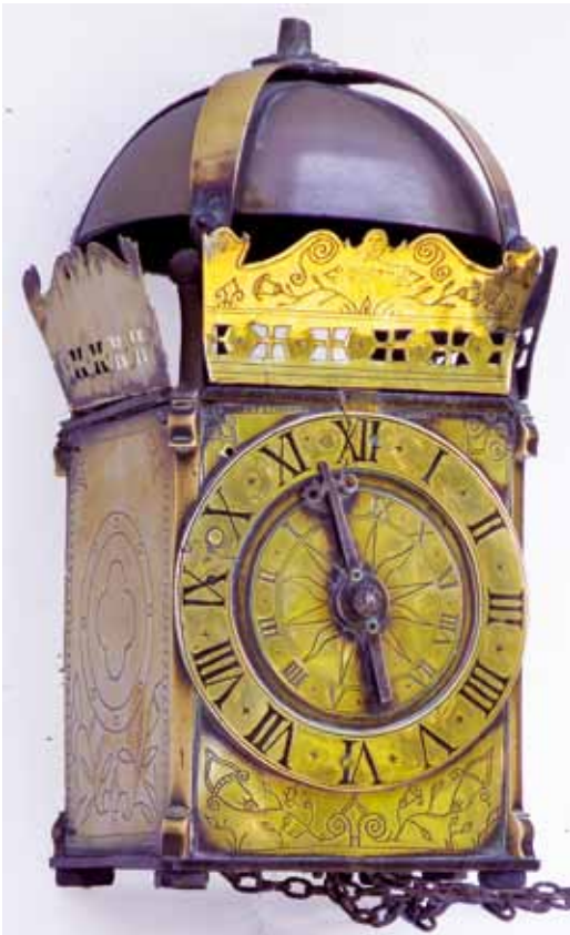
Fig. 15. Unusual brass lantern clock with naively engraved dial, sheet-brass frets and side covers, dated '—77'. (John Robey)
