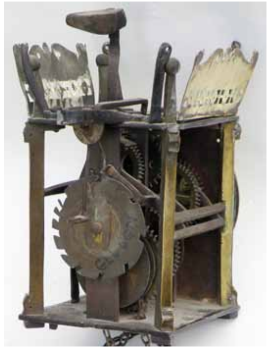
Fig. 16. English movement, but with the strike-work pivoted between angled and buttressed corner pillars. (John Robey)
