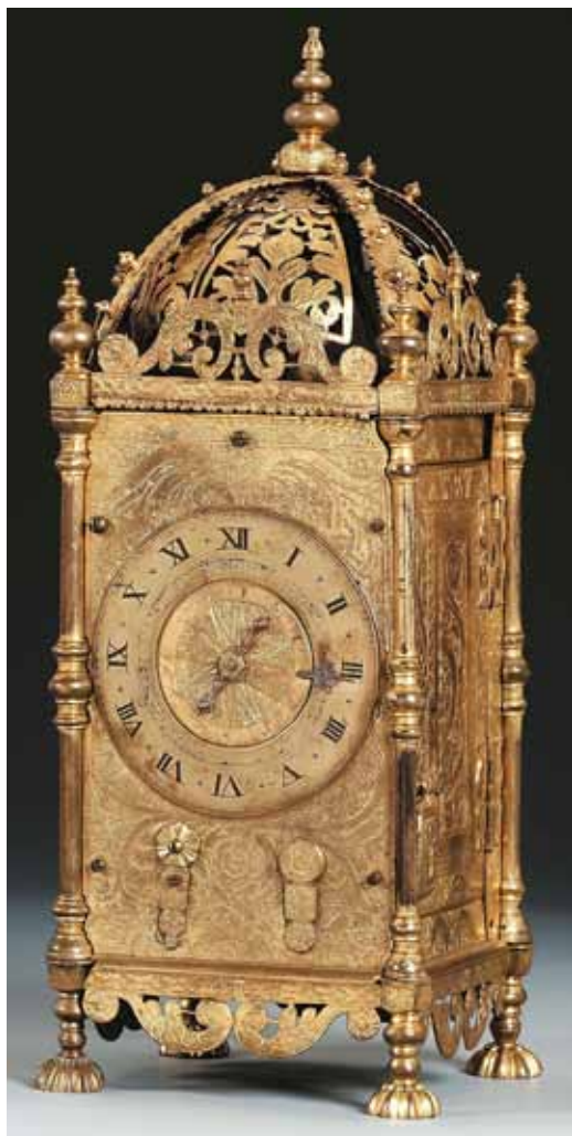
Fig. 20. A very elaborate weight-driven clock with bras corner pillars, feet, finials, bell frame and a separate chapter ring. (© Christie's Images Ltd)
