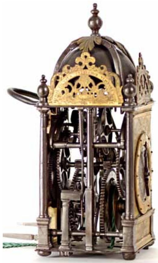
Fig. 27. The frame and wheels of the movement are iron with a vertical hammer shaft. (© Auktionen Dr Crott)
