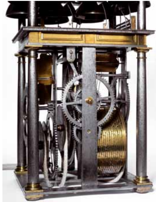
Fig. 23. Movement of the Vallin clock showing the transverse trains with the frame, movement bars and wheels made of iron. (© Trustees of the British Museum)
