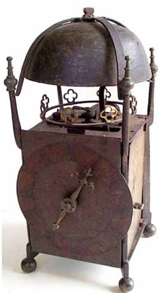
Fig. 17. Unsigned iron lantern clock with a separate iron chapter ring, probably English. (John Hooper)
