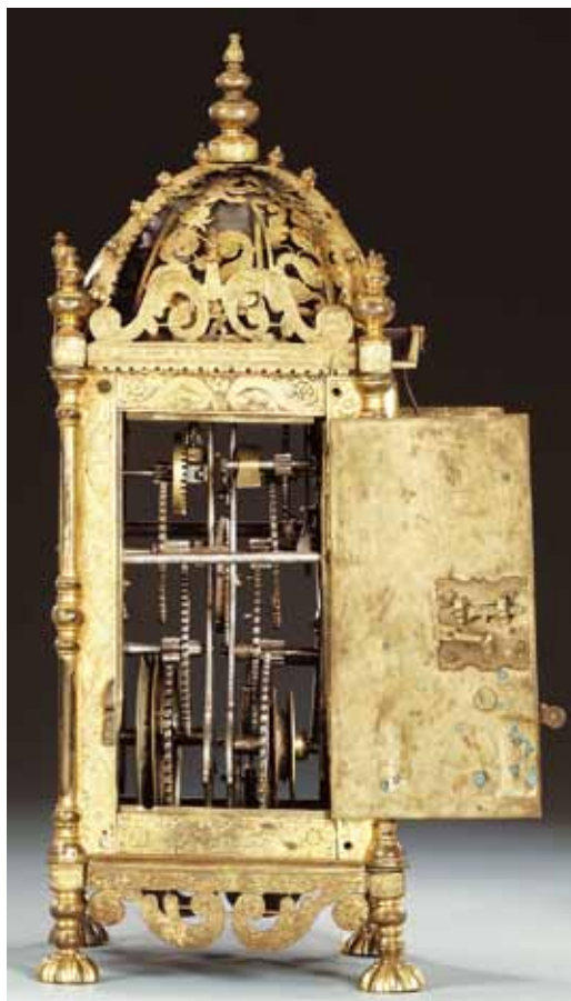
Fig. 21. The partially re-trained iron movement has spiked rope pulleys and a countwheel between two central movement bars. (© Christie's Images Ltd)
