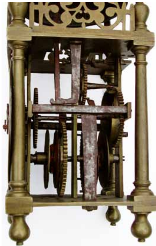
Fig. 34. Movement showing the English style of hammer spring and L-shaped stop. (Brian Loomes)
