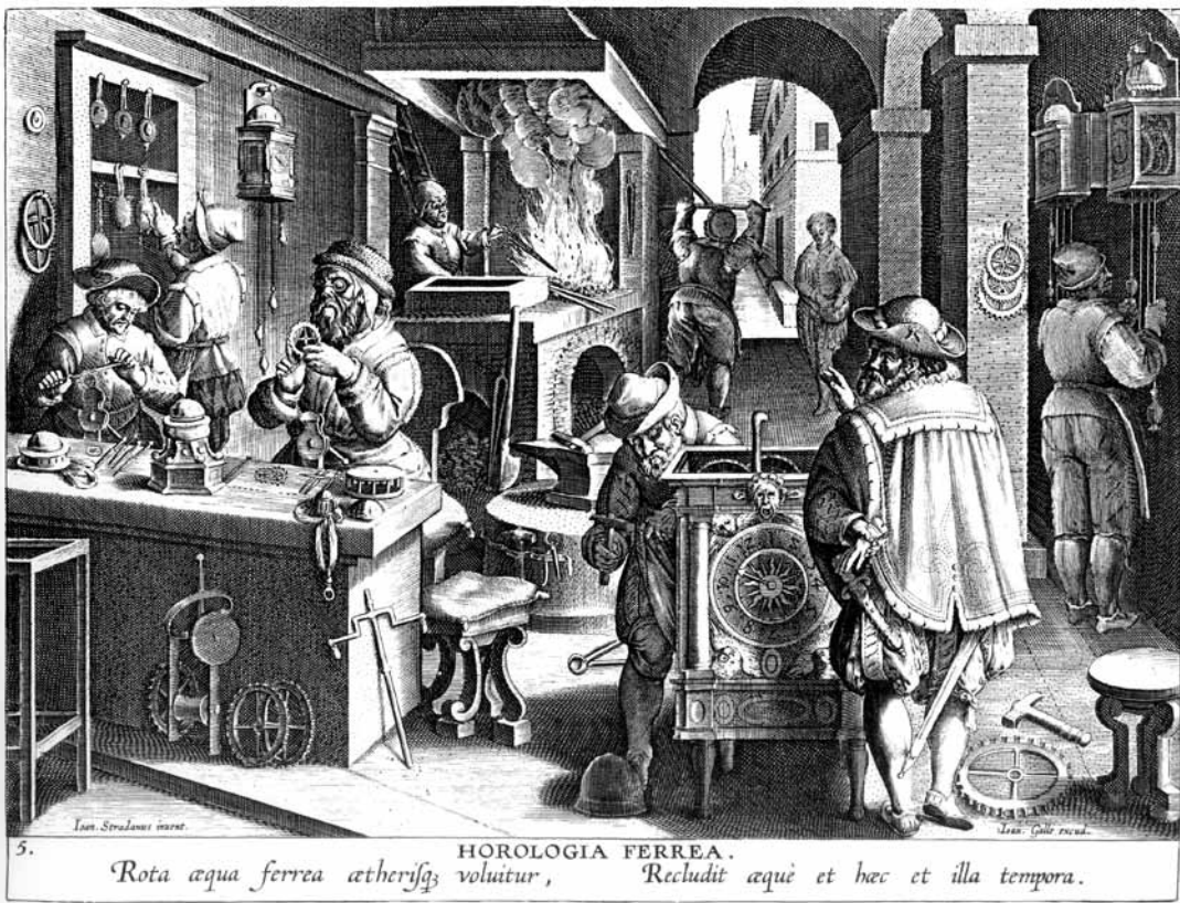
Fig. 31. Engraving of a clockmaker's workshop, by Joan Stradanus, about 1590, dominated by a large forge. The foliot, intended for a turret clock, is fitted upside down.
