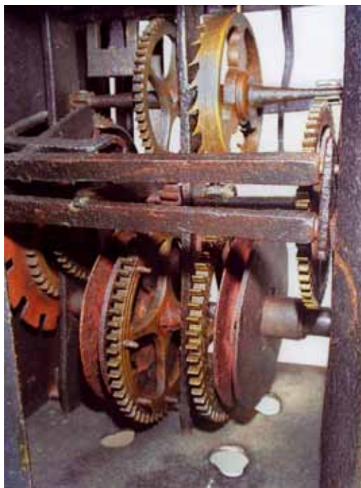
Fig. 18. The movement has brass wheels but with English-style cruciform movement bars of iron. (John Hooper)
