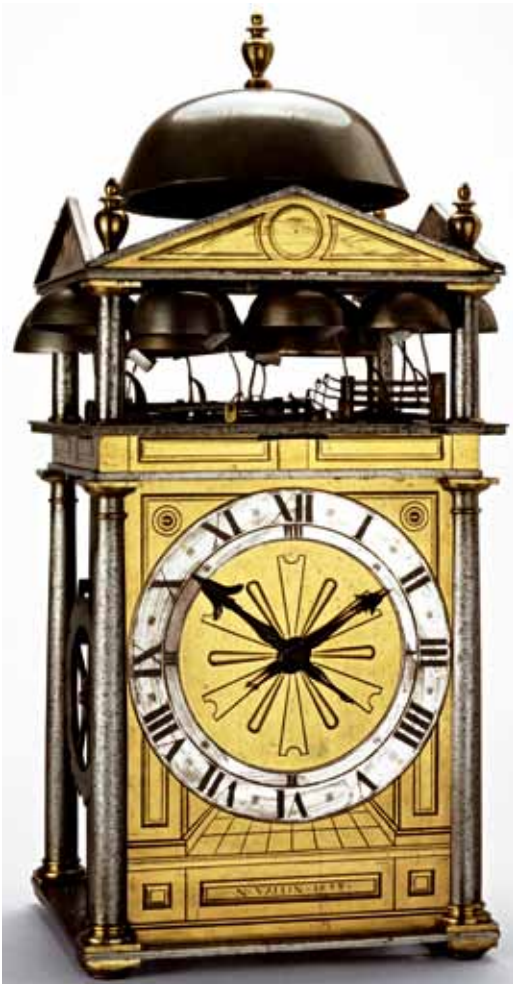
Fig. 22. Carillon clock signed 'N. Vallin 1598' with a brass dial and finials, silvered chapter ring and iron pillars. (© Trustees of the British Museum)
