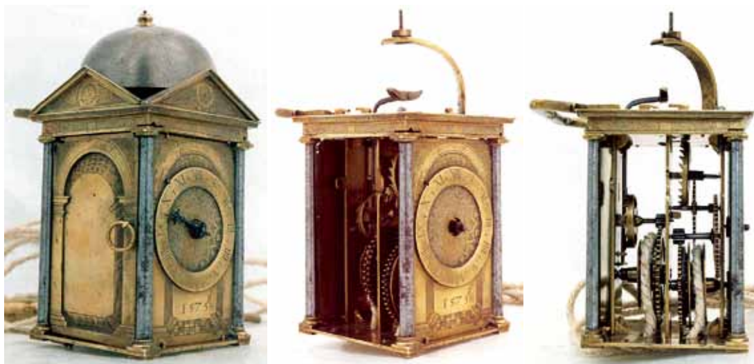
Figs 25a-c. A small weight-driven wall timepiece with alarm from the Low Countries, dated 1575. The wheels and movement bars are of brass. Alarm-setting hand and unlocking lever missing. (Museum van het Nederlandse Uurwerk, Zaandam)
