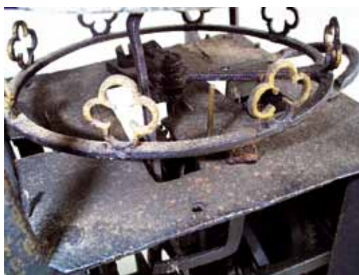
Fig. 19. Original iron balance with eight brass quatrefoils. (John Hooper)
