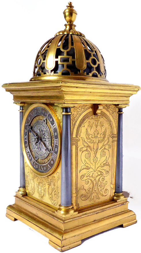
Fig. 2. A late sixteenth-century Flemish spring clock with a gilt-brass base and frieze, iron pillars, pierced bell frame and removable latched side panels. (Richard Newton).
