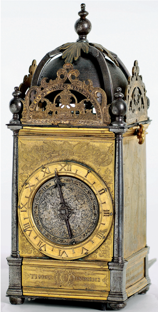
Figs 3-4. A fine late seventeenth-century Renaissance Flemish weight-driven wall clock, with a brass dial, frets and latched side panels, iron wheels, pillars, finials, feet and bell frame. Reconverted back to balance escapement. The hammer shaft is vertical. (© Auktionen Dr Crott).
