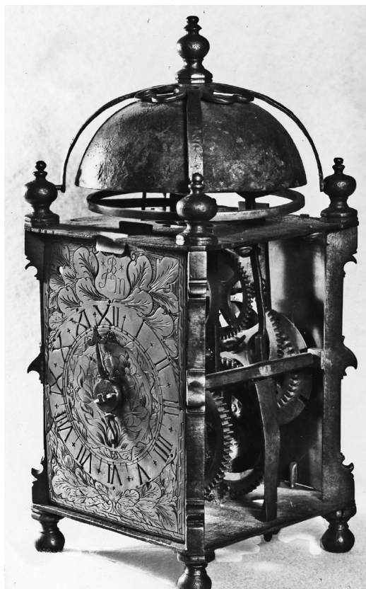
Fig. 1. A mid-seventeenth-century French clock with an iron Gothic-style frame and brass wheels. The dial, bell, bell frame, balance and many other parts are modern, added to make it look like a transitional lantern clock. British Museum BM1958, 1006, 2096. (© Trustees of the British Museum)
